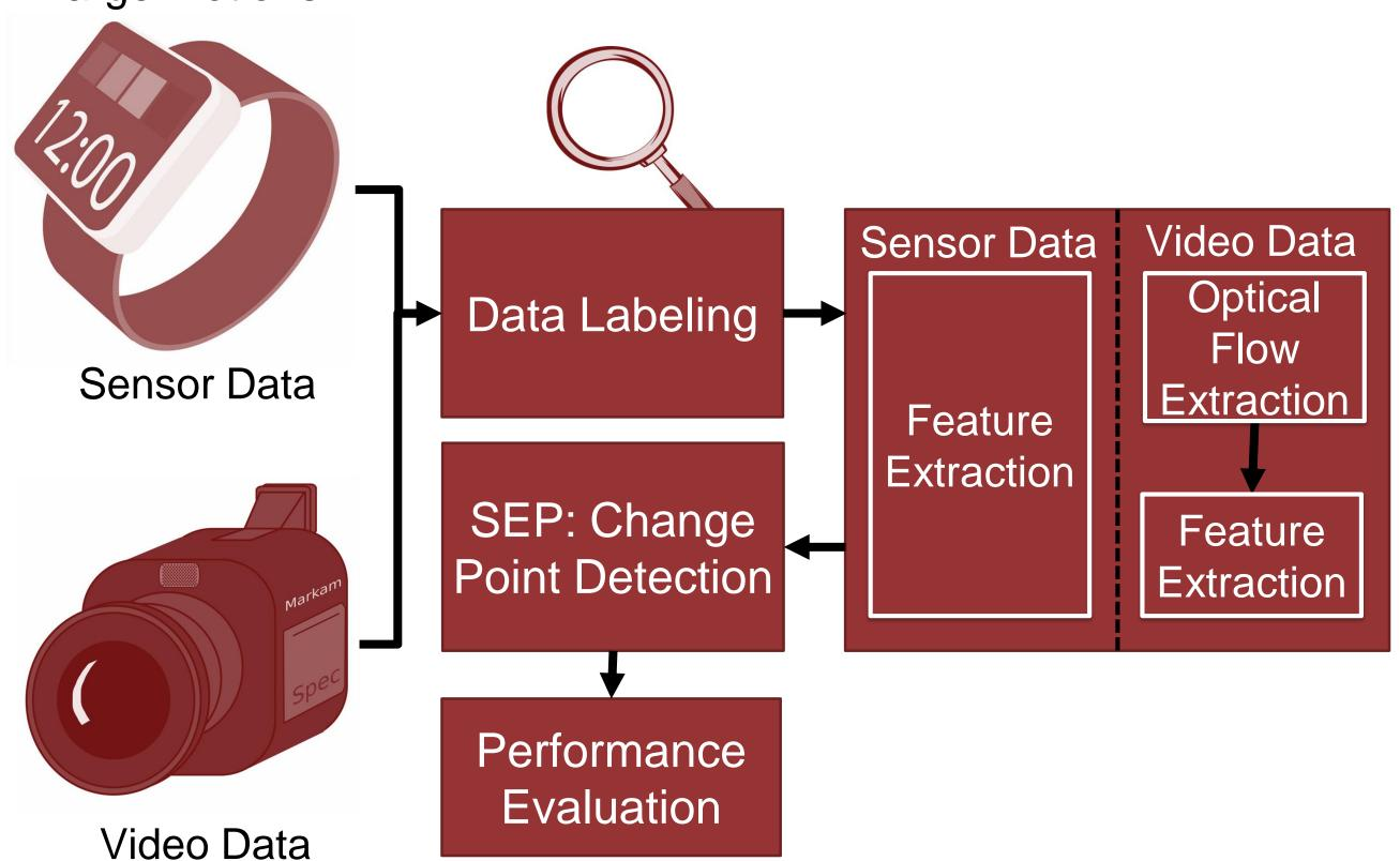
**Sensor Data:** Yaw, Pitch, Roll, Rotation (X,Y,Z), Acceleration (X,Y,Z) Sensor Data Feature Extraction: Mean, Max, Min, Stdev, Range for 10 second window duration
