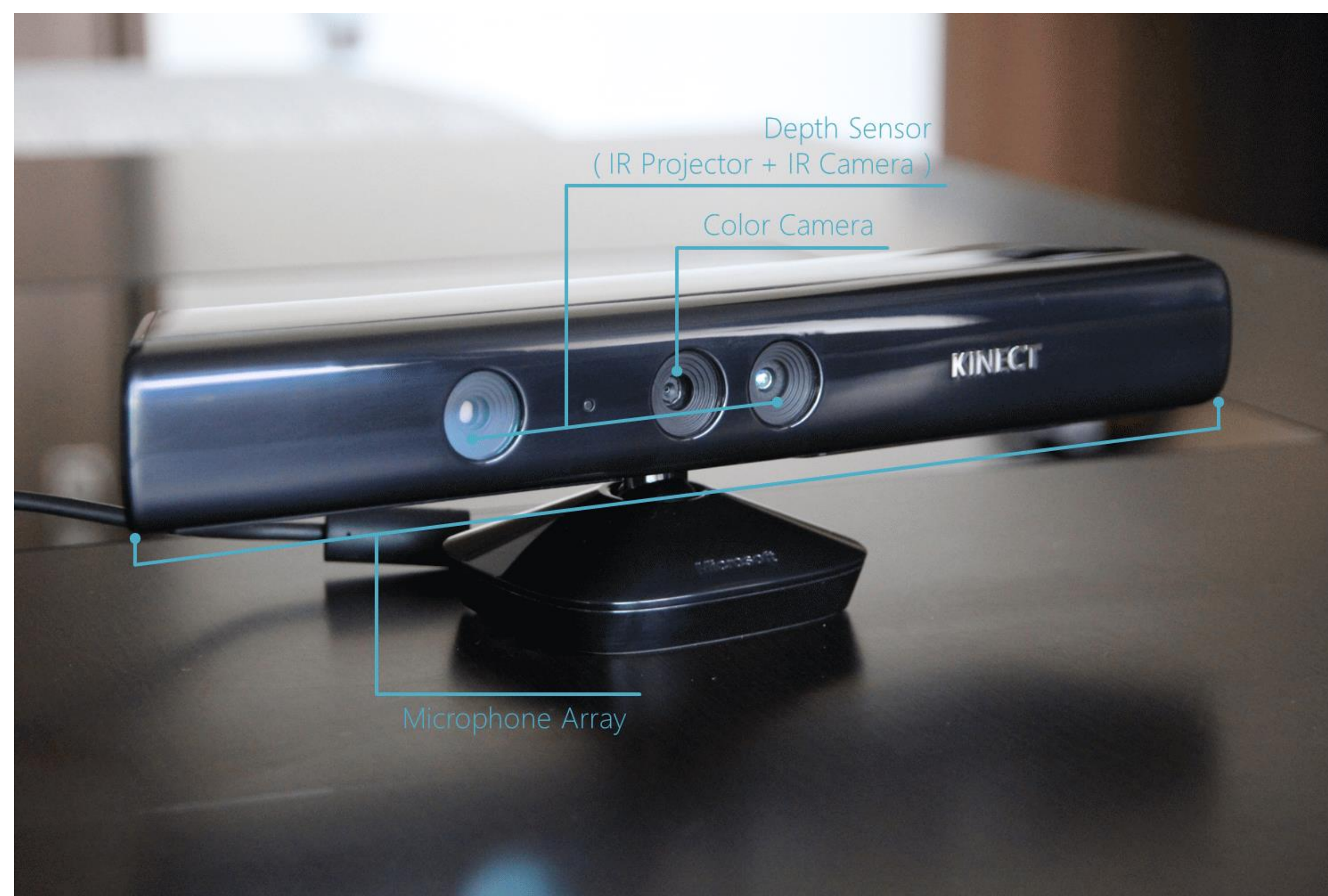
Figure 2: Image of the Kinect V1 and its various sensors
