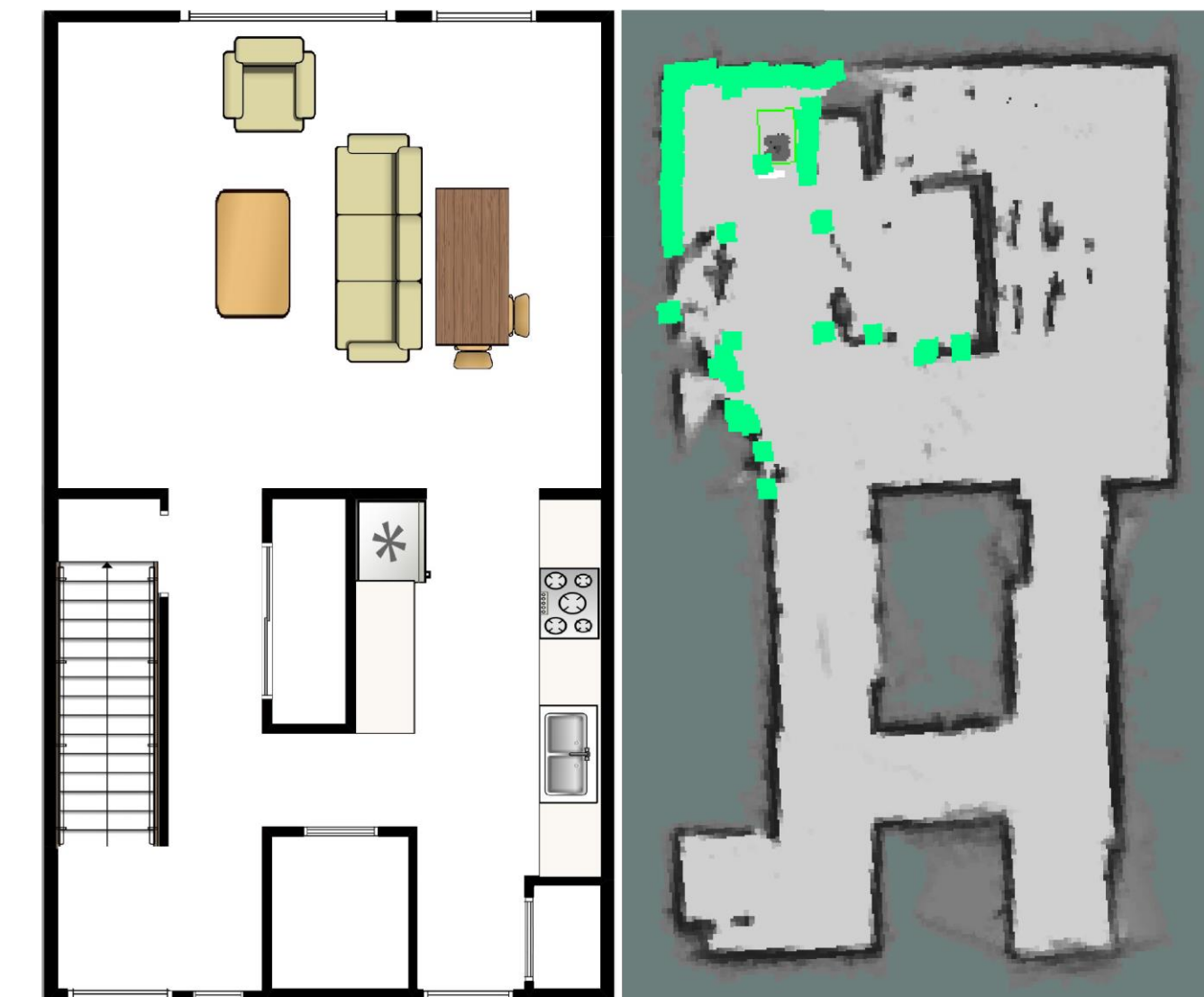
Figure 5. Cartographer map of the smart apartment, green dots show current lidar scan, the green rectangle represents the robot footprint
